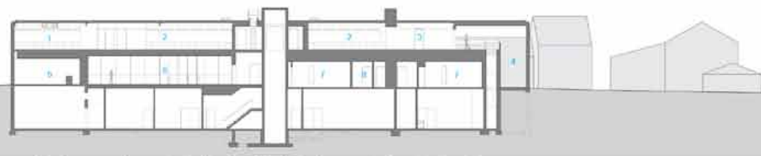
1. conference room 2. open office 3. office 4. porch 5. gift shop 6. entry portico 7. workshop 8. media center section A-A'
